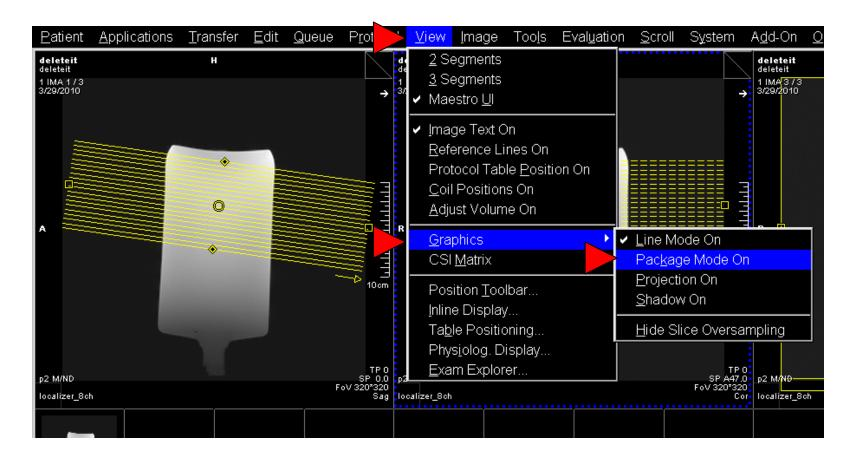
To switch from lines to a box, Click on "View" then "Graphics" and last "Package Mode On". To switch back to lines Click on "Line Mode On".
