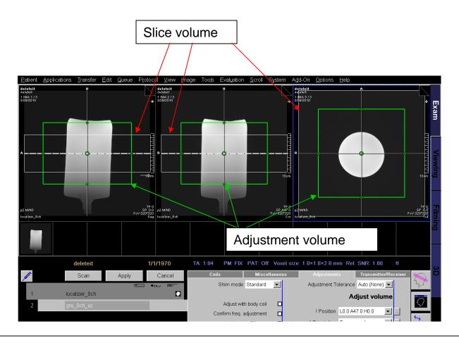
Green box indicates "Adjust volume on". If you do not typically use the 'Adjust volume on", turning it off will shim to your slice volume, which is represented by the gray rectangular box in this example.
