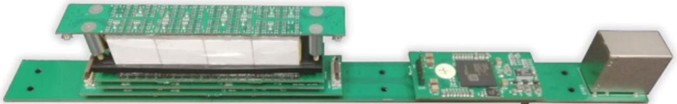
Figure 1. A single PET modules with scintillation crystal, photodetector, and preamplifiers on the left. The FPGA, power components, and connector are on the right. Two opposing modules were used to evaluate MRI compatibility.
