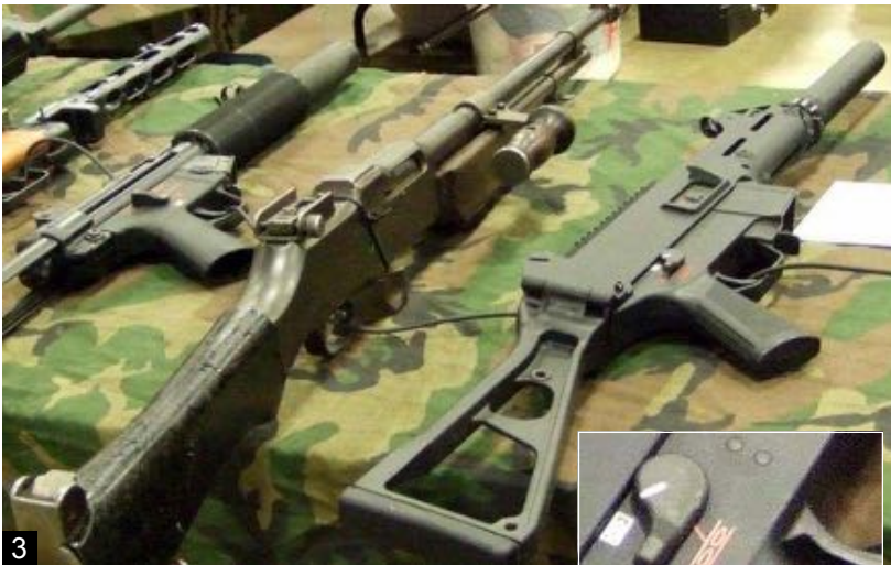
This selector switch has 3 positions: safe, semiautomatic, and automatic. The receivers in Photo 6 are similarly equipped (4 positions: safe, semiautomatic, burst, and automatic).
